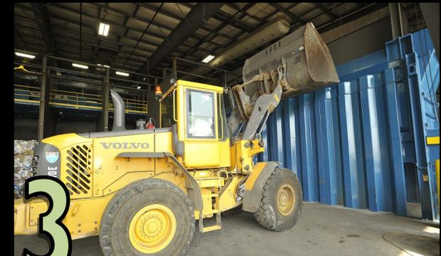
**3** The material is mixed by the loader and placed into a metering bin to start the sortation process.
