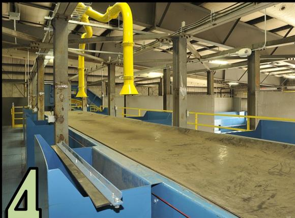
**4** First line is the 'pre-sort' line where scrap metals, shredded office paper, and other bulky items are removed from the conveyor line. At the end of this line, materials are separated by fibers (papers, cardboard) and containers (plastics, metals, cartons) for additional sortation.
