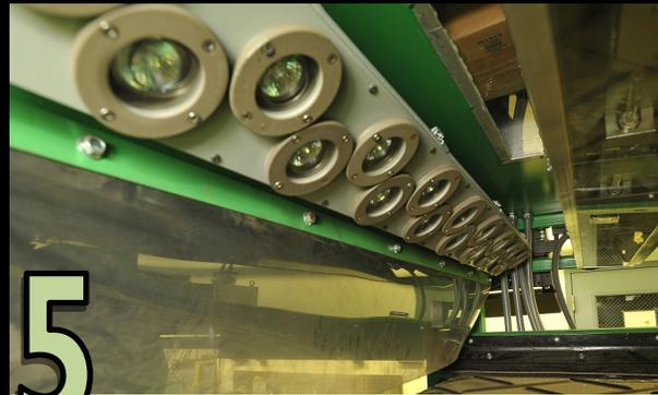
**5** Pictured above is one of four green machines, each machine optically sorts each different type of plastics (#1 PET, #2 HDPE Colored and Natural), and one is designated for cartons. Further down the line, a magnet is used to sort out steel/tin cans and then an eddy current machine is used to separate aluminum cans.
