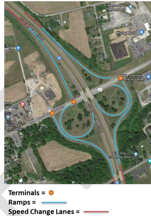
Figure 8: Terminal, Ramp, and Speed Change Lane
