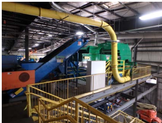
Fourth Green Eye : enables the system to sort and recycle cartons
