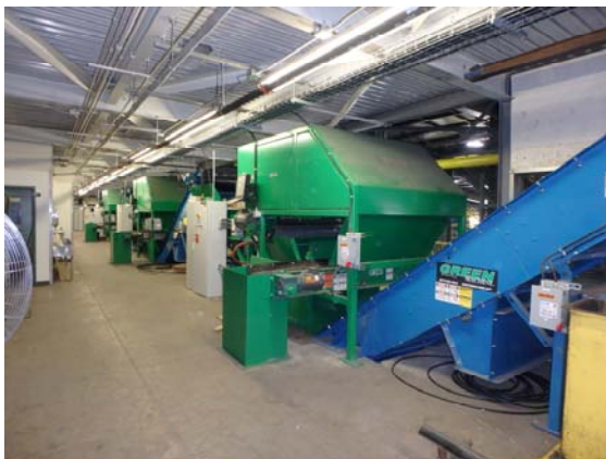
Series of three Green Eyes for sorting plastic
