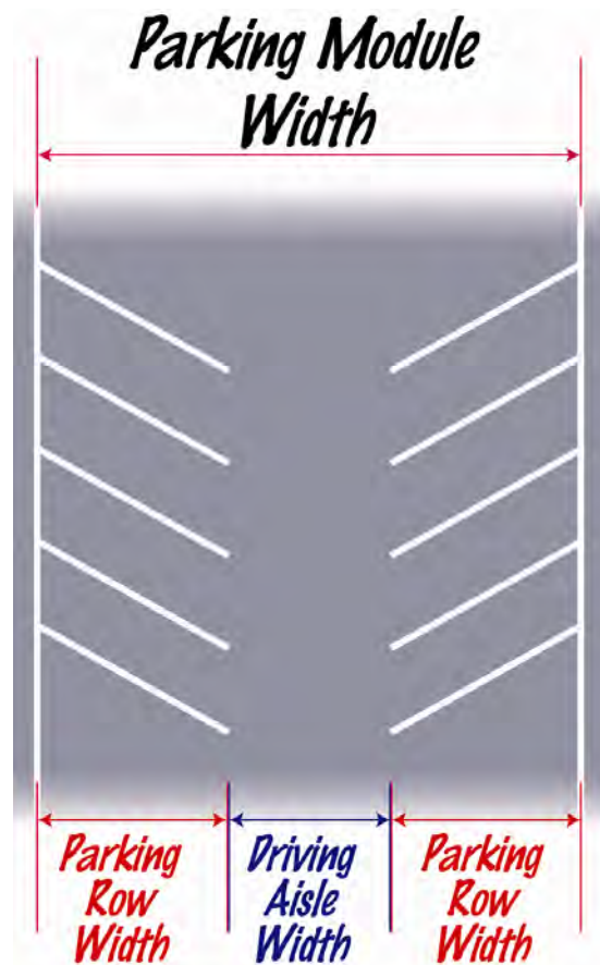
Illustration 7101.C - Off-Street Parking Design Standards
