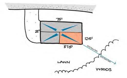
i.e. Impervious Area of Roof Quarter Flow path of 50'
