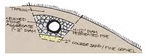
When installing a level spreader pipe, first dig a shallow trench for the pipe. Downspout disconnects can be connected to this pipe. The trench should run evenly along a slope contour. The trench should be bedded with about 2" of course sand, and contain uniformly crushed stone, pieces 1"-3" in diameter. Level spreaders should have a **minimum length of 10 feet**, for impervious areas around 500 sq ft. Add 10-30 additional feet for larger impervious surfaces.
